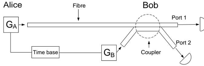
**Figure 1** The schematic diagram of the quantum cryptosystem using an optical coupler. Alice's (or sender's) signal generator is labeled by  $G_A$ ; Bob's (or receiver's) is labeled by  $G_B$ .
