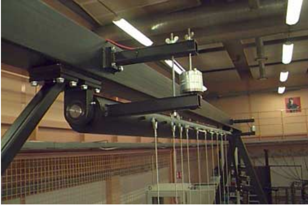
Figure 4: Releasing mechanism with electrical magnets.
