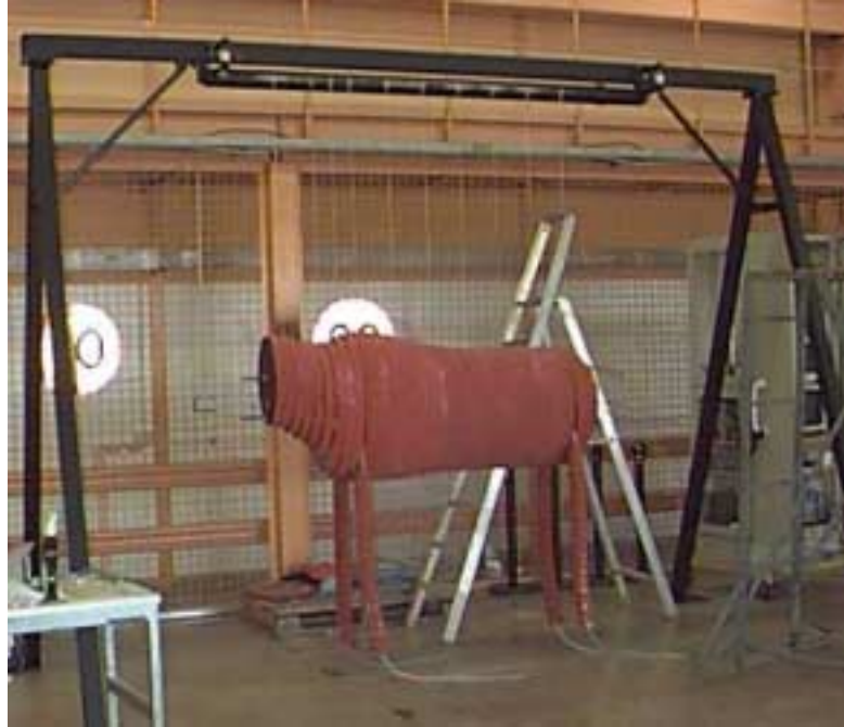
Figure 11: Dummy hanging from the releasing frame.
