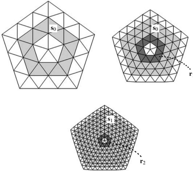
Figure 4: The surfaces  $\mathbf{s}_0, \mathbf{s}_1$  (light gray) and the surface rings  $\mathbf{r}_1, \mathbf{r}_2$  (dark gray) generated by the algorithm of Loop from an initial control net  $\mathcal{C}_0$  with one irregular vertex of valence  $n = 5$  (schematically).
