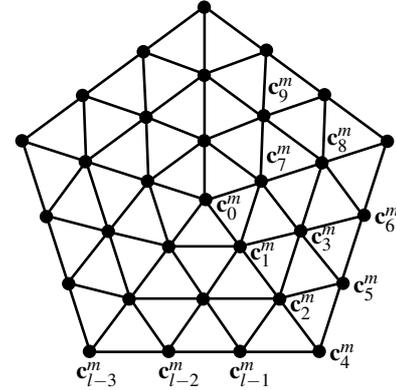
Figure 5: A numbering for the control points of  $\mathcal{C}_m$  for the algorithm of Loop.
