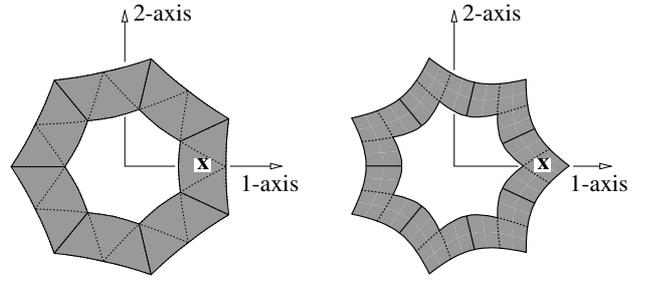
Figure 6: The characteristic map of the algorithm of Loop (left) and the algorithm of Catmull-Clark (right) for an irregular vertex of valence 7. The dashed lines show the boundaries of the polynomial pieces. The solid lines show the boundaries of the segments, especially the normalized segment  $\mathbf{x}$ .
