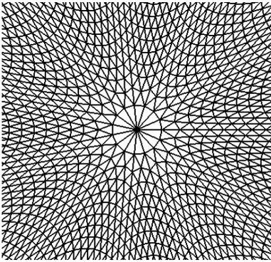
Figure 7: Polar artifacts for the algorithm of Loop at an irregular vertex of valence  $n = 15$ .
