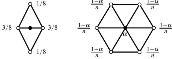
Figure 1: The stencils of the algorithm of Loop at a vertex of valence  $n$ , where  $\alpha = 3/8 + (3/8 + \cos(2\pi/n)/4)^2$ .
