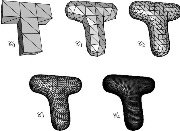
Figure 2: The initial triangular net  $\mathcal{C}_0$  (top left) and the nets  $\mathcal{C}_1, \dots, \mathcal{C}_4$  of the first four iteration steps of the algorithm of Loop.
