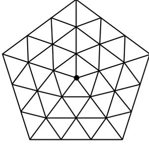
Figure 3: An initial triangular net  $\mathcal{C}_0$  with an irregular vertex of valence  $n = 5$  (marked by  $\bullet$ ) surrounded by three rings of regular vertices for the algorithm of Loop.
