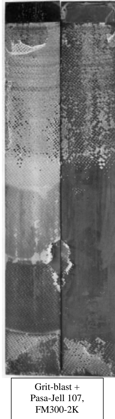
Figure 8 Fracture surface of failed wedge test indicating the relative areas of adhesion failure for the FM300-2K bonded titanium samples pre-treated with grit-blasting and Pasa-Jell 107.
