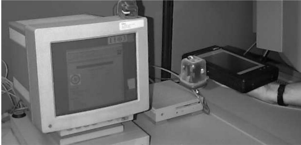
Figure 7: Home-made ir units allow cross-platform communication.
