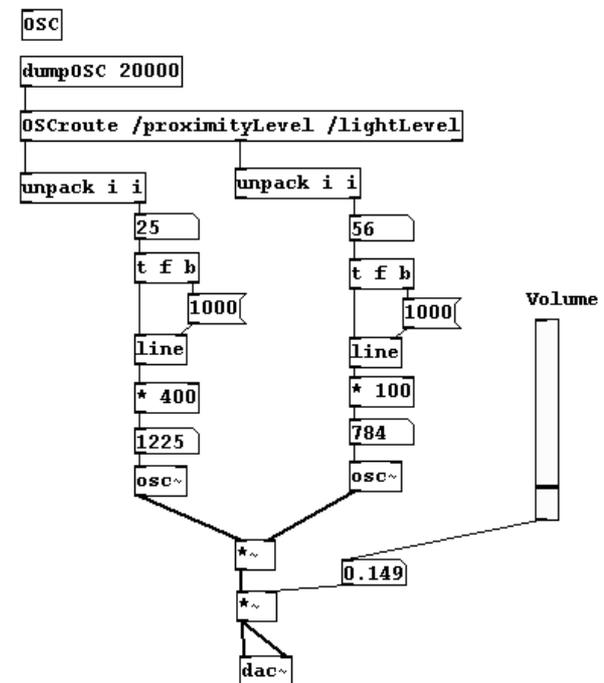
Figure 10: Pure Data implementation of a robot theremin.
