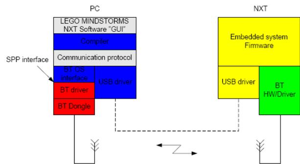
Figure 2: Communication block diagram, from (Lego Group, 2006a).
