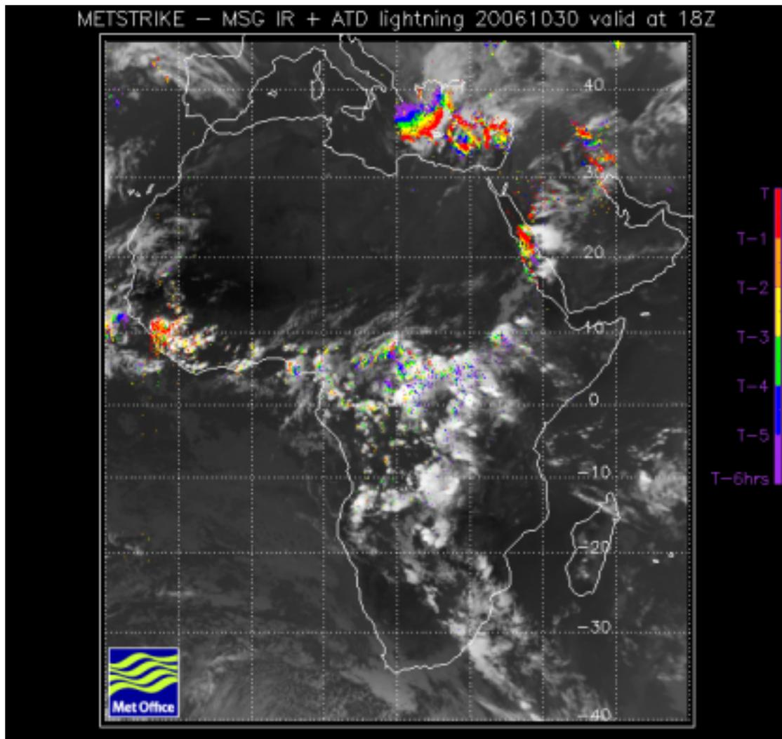
Fig. 4.1 Current ATD superimposed on Meteosat MSG cloud picture – a possible product for supply to Africa with ATDNET in future. Here the latest observations are in red and the observations 6 hours earlier are in purple.
