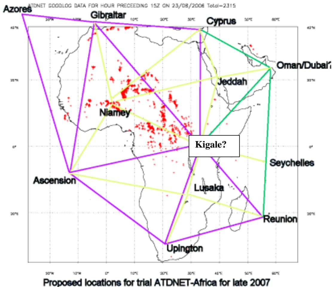
Fig. 2.4 Possible location of ATDNET outstations for good coverage of Africa., superimposed on thunderstorms detected with new ATDNET using European stations only in August 2006. Purple lines indicate the stations that are expected to be established first and the green and yellow lines join to potential sites that have not yet been approached.
