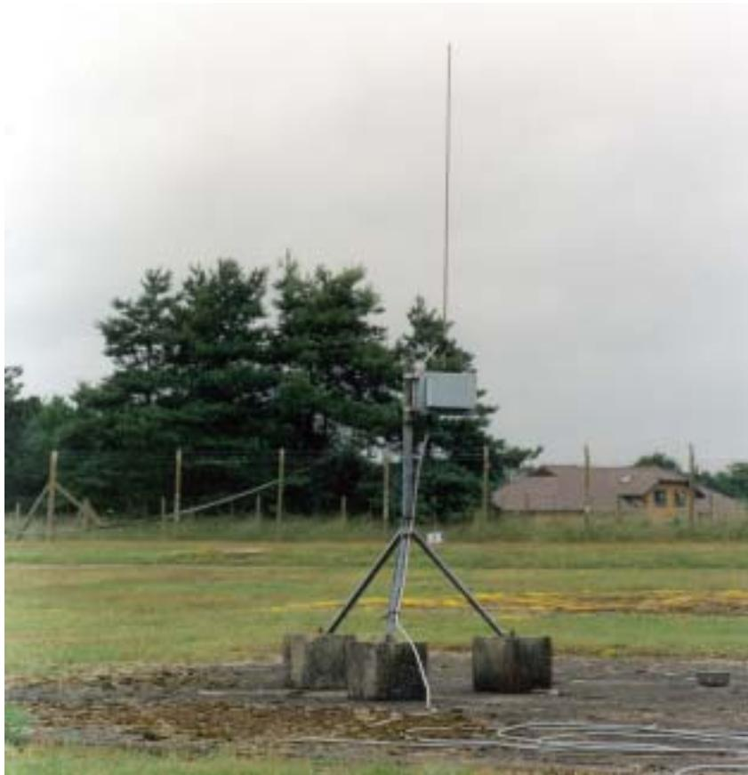
Fig. 2.1 ATD whip antenna used for observations at 10 kHz or 13.6 kHz [frequency can be changed using software]
