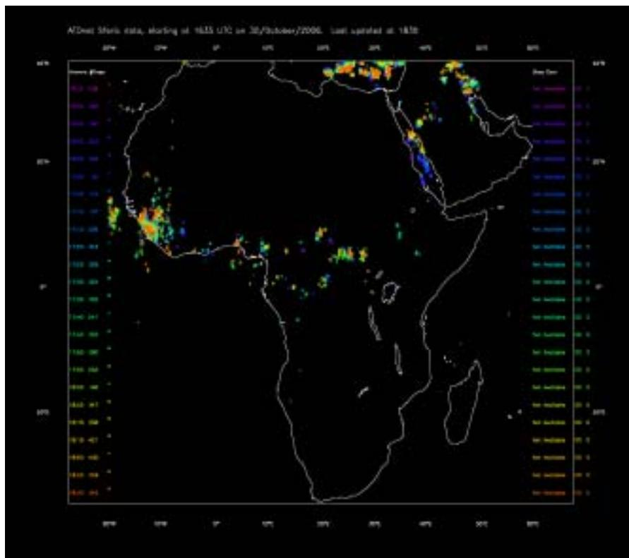
Fig. 3.3 (b) ATDNET flash locations for Africa displayed on Upper Air Team workstation having completed processing by the flash location processor and storage in the Logical Data Store.
