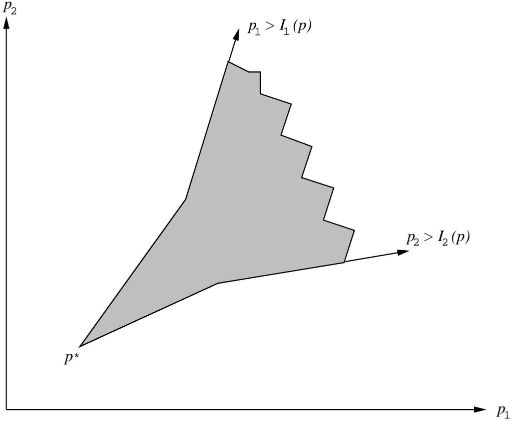
Figure 1: The interference constraints under MPA. The shaded region denotes the set of feasible power vectors under MPA for a system of two users and two base stations. The breakpoints of the constraints occur when the base station assignment changes. We observe that the set of feasible power vectors is nonconvex.
