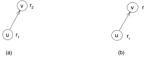
Figure 3.11: (a) (u, v) is natural; (b) (u, v) is natural if r_i has no self-loop in RTG.
