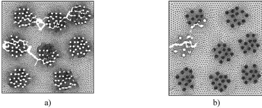
Figure 10. Cluster microstructures: (a) Fine, step 6,  $u = 5.99E-03$  mm, (b) Coarse, step 6.
