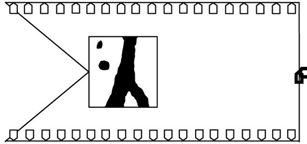
Figure 4. Loading scheme of the mesomodel.
