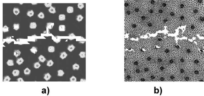
Figure 6. Comparison of the crack path simulated in the artificially designed random coarse microstructure with the use of different numerical approaches: (a) MPE, element softening (Mishnaevsky et al., 2003b), (b) automatically generated FE mesh, element elimination.
