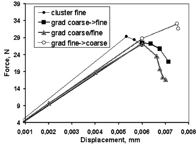
Figure 12. Force-displacement curves for the simulated microstructures.
