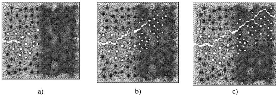
*Figure 9.* Layered microstructure 1 (coarse  $\rightarrow$  fine): (a) Step 8,  $u = 6.38E-03$  mm, (b) step 14,  $u = 6.75E-03$  mm, (c) step 26,  $u = 7.13E-03$  mm.
