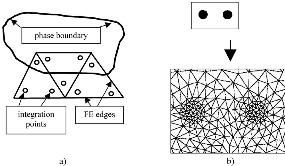
Figure 2. Schemes: Multiphase finite elements (a) and automatic FE mesh generation from microstructures (b)
