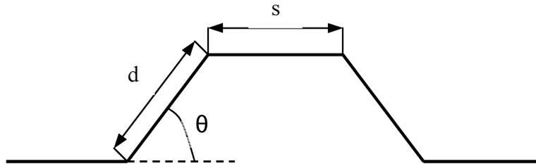
Figure 16. Schematization of the crack deviation according to Suresh (1998).
