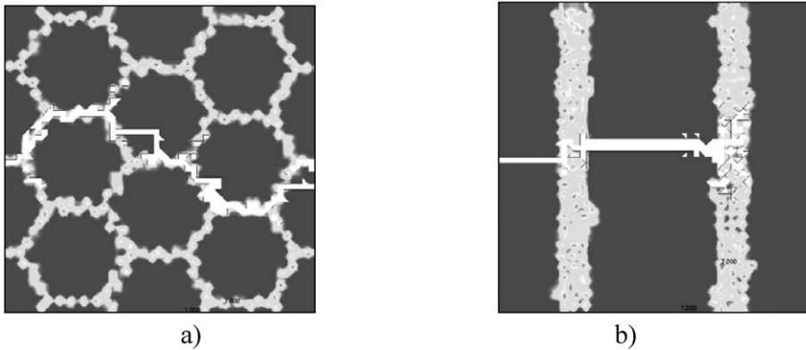
Figure 11. Crack path in net-like microstructures (a) and band-like microstructure (b) (given here for comparison purposes) (Mishnaevsky et al., 2003b).
