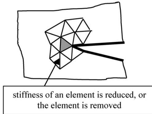
Figure 3. Scheme: Elimination or softening of a finite element.
