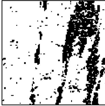
*Figure 1.* Discretized micrograph of high speed steel HS6-5-2 (Mishnaevsky et al., 2003b). The black areas represent primary carbides, the white area is the ‘matrix’. Region dimension  $100 \mu\text{m} \times 100 \mu\text{m}$ .
