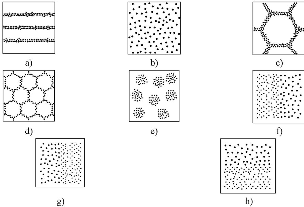
Figure 5. Artificial arrangements of primary carbides considered in this work: (a) band-like, (b) random, (c) net-like coarse, (d) net-like fine (Mishnaevsky et al., 2003b), (e) clustered, (f–h) layered (3 different orientations).
