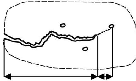
Figure 13. Scheme: Crack path variations due to the microcracks.
