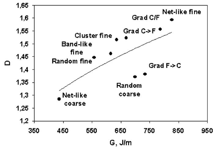
Figure 14. Fractal dimension D plotted versus the calculated fracture energy.
