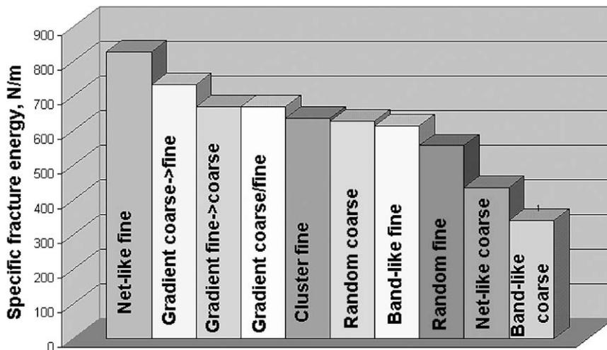
Figure 15. Comparison of fracture resistance of different artificial microstructures.
