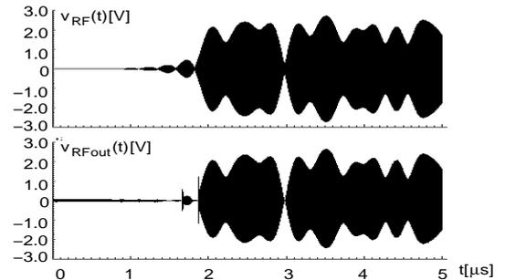
Figure 6. The original and output WCDMA RF signal
