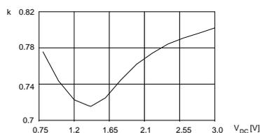
Figure 8. Non-constant  $V_{out}/V_{DC}$  ratio in a class E PA
