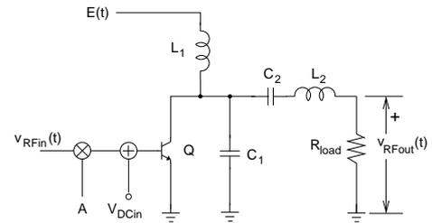
Figure 5. Class E PA with EER applied
