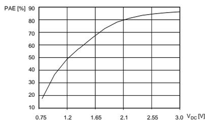
Figure 9. PAE dependence on the supply voltage
