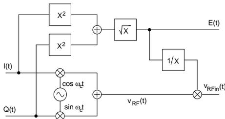
Figure 4. Linearization circuit
