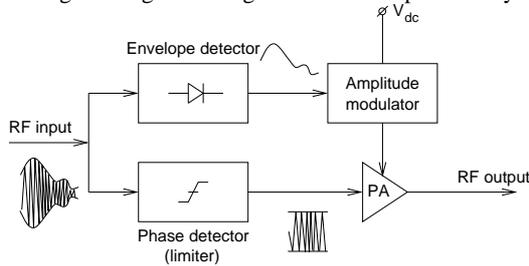
Figure 2. Block diagram of the EER principle
