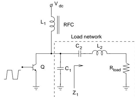
Figure 1. Basic circuit diagram of a class E PA
