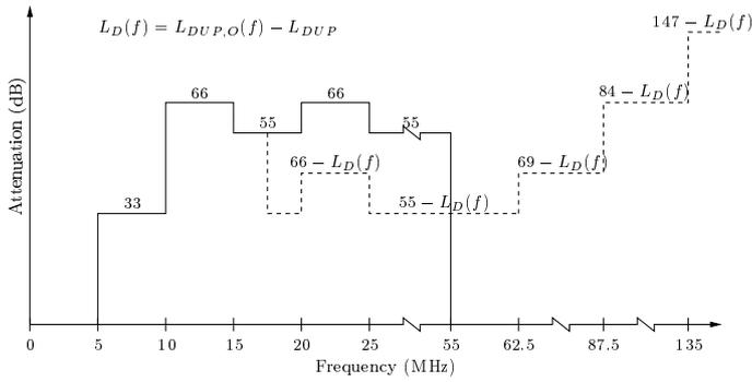
Fig. 1. Worst case adjacent channel attenuation requirements as a function of frequency offset from the center frequency of the desired channel [3]. The solid line indicates the attenuation requirements within the UMTS downlink band, while the dashed line indicates the out-of-band requirements.
