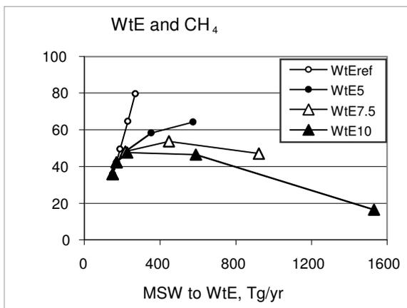
Fig. 3. Impact of WtE capacity on methane emission from landfills. Values plotted for 2000, 2005, 2010, 2020 and 2030 for each scenario.
