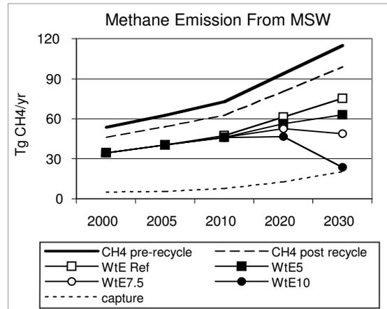
Fig. 2. Impact of WtE growth on net methane emission from MSW. The solid line, potential maximum, is included for reference only.
