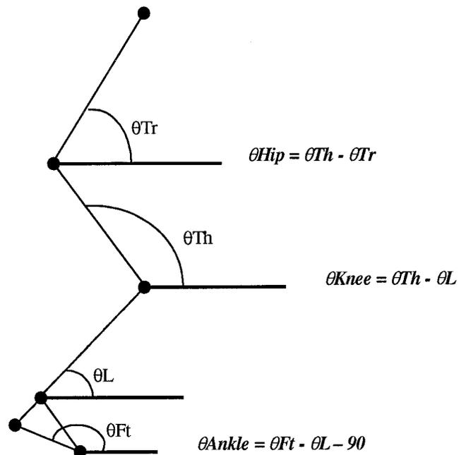
**Figure 1**—Convention used for calculation of segmental and joint angles from marker coordinate data.
