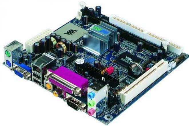
Figure 3.2: EPIA M10000 system platform
