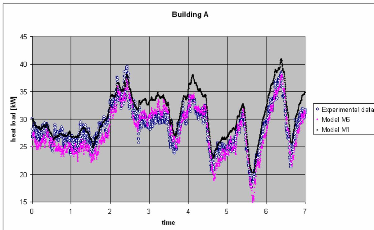
Figure 2. Experimental data and simulation models M1 and M6.
