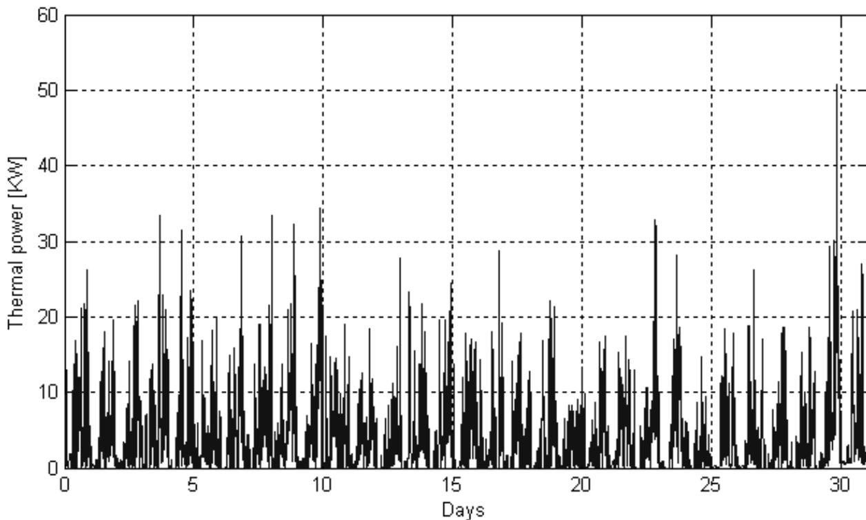
Figure 3. Daily thermal power consumption of domestic warm water during a month.
