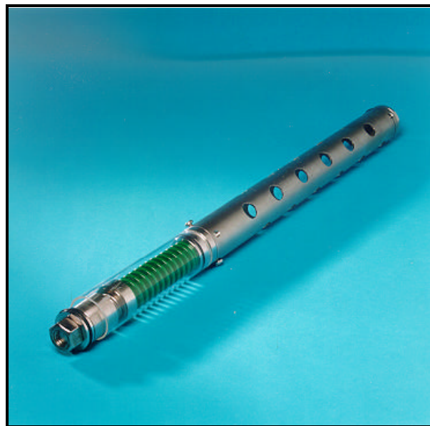
Figure 19: Self stressed tube for combined environment/stress testing
