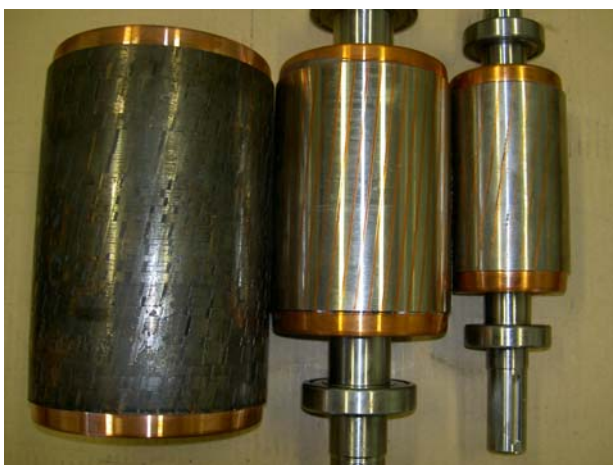
Fig. 3 – View of copper rotors for the considered motors
