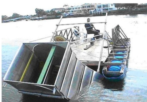
Fig. 17: CFWT in diffuser mounted in front of motorized barge
