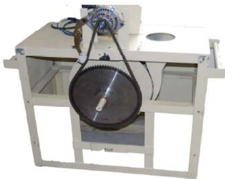
Fig. 12: Pico hydro turbine system
