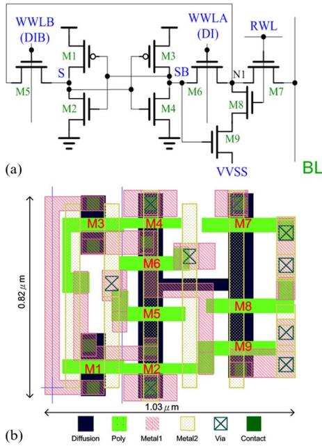
Fig. 1. (a) Schematic of the disturb-free 9T cell [19] and (b) layout of the 9T cell in UMC 40-nm low-power (40LP) CMOS technology.
