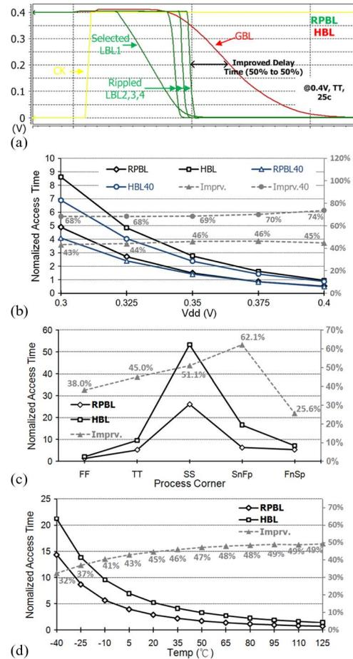
Fig. 3. Comparison of the conventional HBL and the proposed RPBL scheme in UMC 65LP CMOS technology: (a) pertinent sensing waveforms at 0.4 V, TT, 25 °C; (b) Read access delay ( $T_a$ ) versus VDD at TT, 25 °C, also shown for comparison are the 40LP results (labeled HBL40, RPBL40, and Imprv.40); (c)  $T_a$  versus process corner at 0.4 V, 25 °C; and (d)  $T_a$  versus temperature at 0.4 V, TT.
