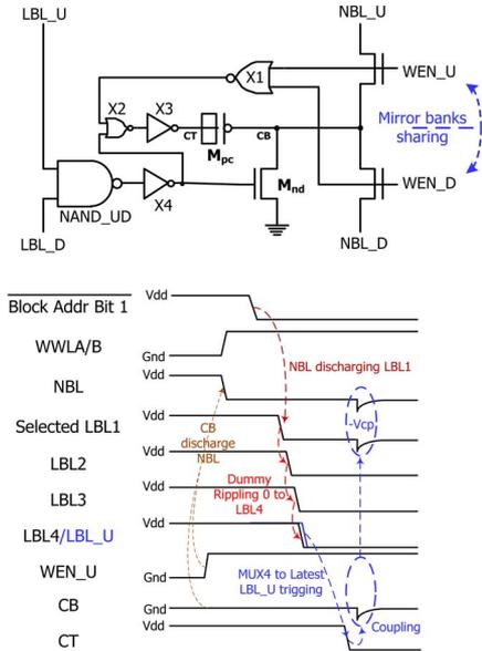
Fig. 5. Ripple-initiated NBL circuitry and pertinent timing diagram during Write operation.  $M_{pc}$  is the boosting capacitor implemented with PMOS.
