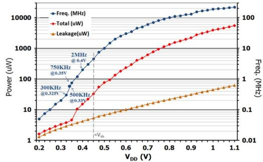
Fig. 9. Measured maximum operation frequency, the leakage power, and total power versus  $V_{DD}$ .
