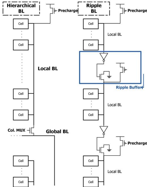
Fig. 2. Conventional hierarchical BL (HBL) scheme and proposed ripple BL (RPBL) scheme. The ripple BL scheme isolates each LBL segment through ripple buffer insertion.
