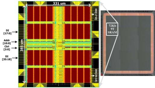
Fig. 6. Die photo (right) and layout view (left) of the 72-Kb test chip in UMC 40-nm low-power (40LP) CMOS technology.
