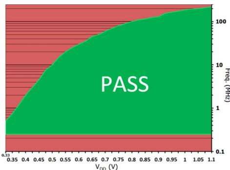
Fig. 10. Measured frequency-voltage Shmoo plot of the 72-Kb RPBL test chip.
