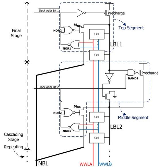
Fig. 4. Details of precharge circuits for the top LBL segment and middle LBL segment, and coupling of negative bit-line (NBL) transient pulse into the selected LBL segment.
