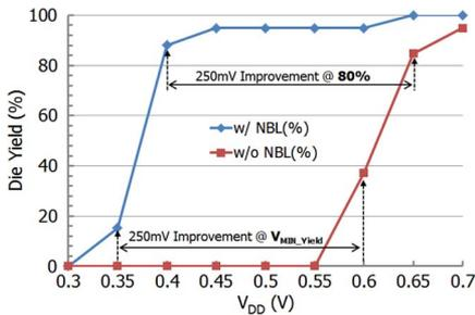
Fig. 7. Measured error-free full functionality die yield versus  $V_{DD}$  at room temperature. A total of 59 dies are measured.
