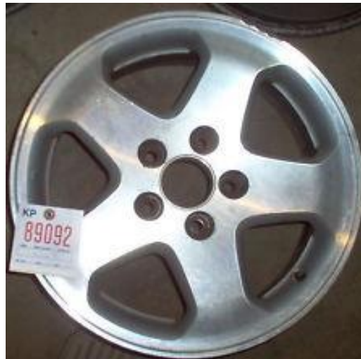
( C ) Actual view of the wheel after optimization and removing the unwanted material.
