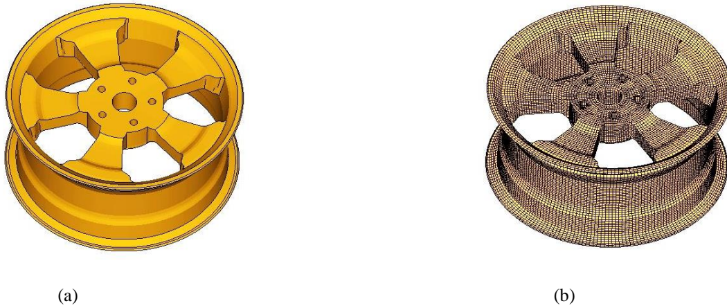
Fig.7 (a) CAD model and optimized design of the wheel rim (b) Mesh model of the wheel rim for finite element analysis.
