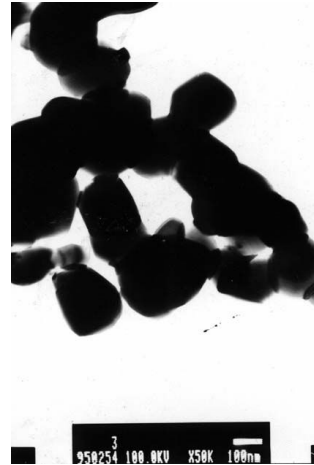
Fig.3. (b) TEM of conventional powders average particle size 600nm
