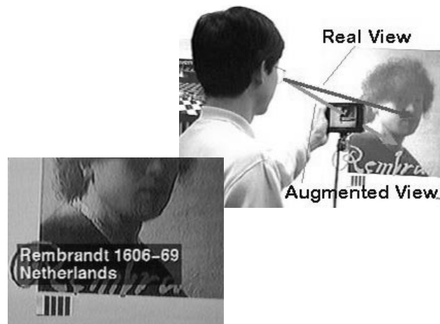
Figure 1: In Rekimoto and Nagao's NaviCam system (1995), a handheld device recognizes tagged objects and then overlays context-sensitive information.
