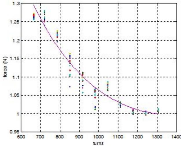
Figure 15. Force vs. turns for an actual solenoid
