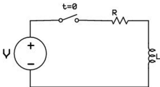
Figure 1. Equivalent Circuit
