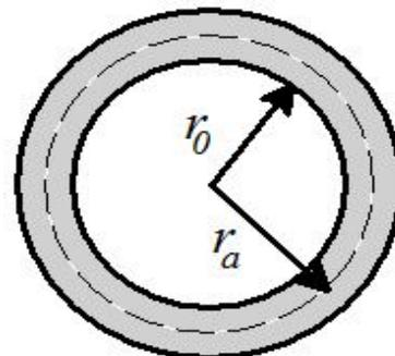
Figure 5. Coil radius vs. average turn radius
