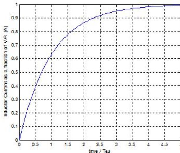
Figure 3. Current through the inductor
