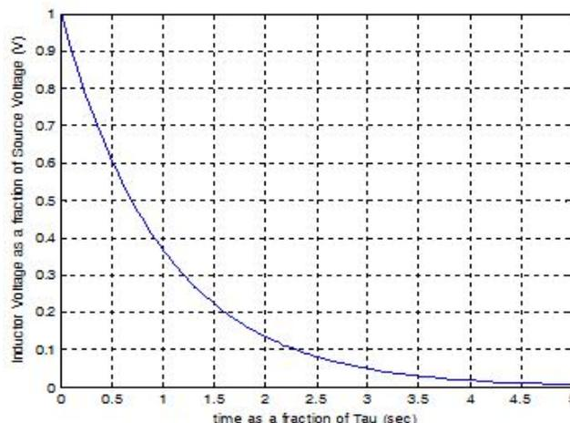
Figure 2. Voltage across the inductor
