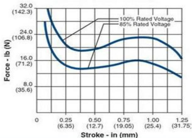
Figure A.1. Force Stroke Curve for an AC Solenoid
