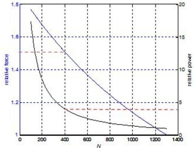
Figure 9. Relative force and power vs.  $N$
