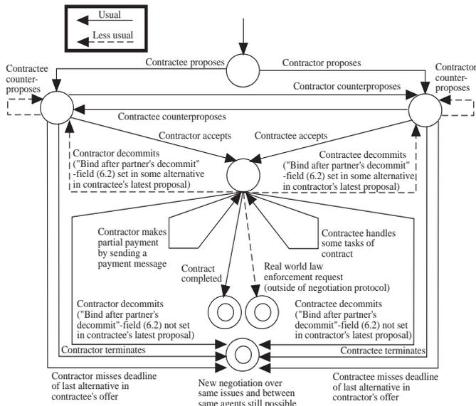
Figure 2: State transition diagram of a single negotiation.
