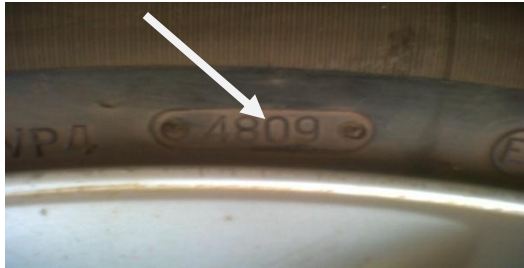
Figure 1. Diagram of a tire showing the manufactured date
