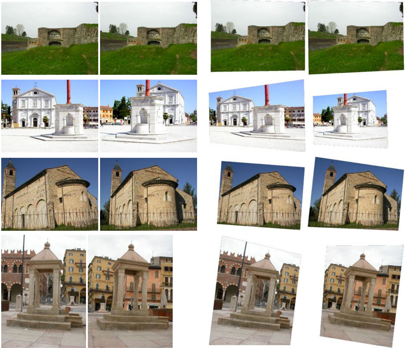
Figure 4. Original uncalibrated pairs (left) and Quasi-Euclidean rectification (right).
