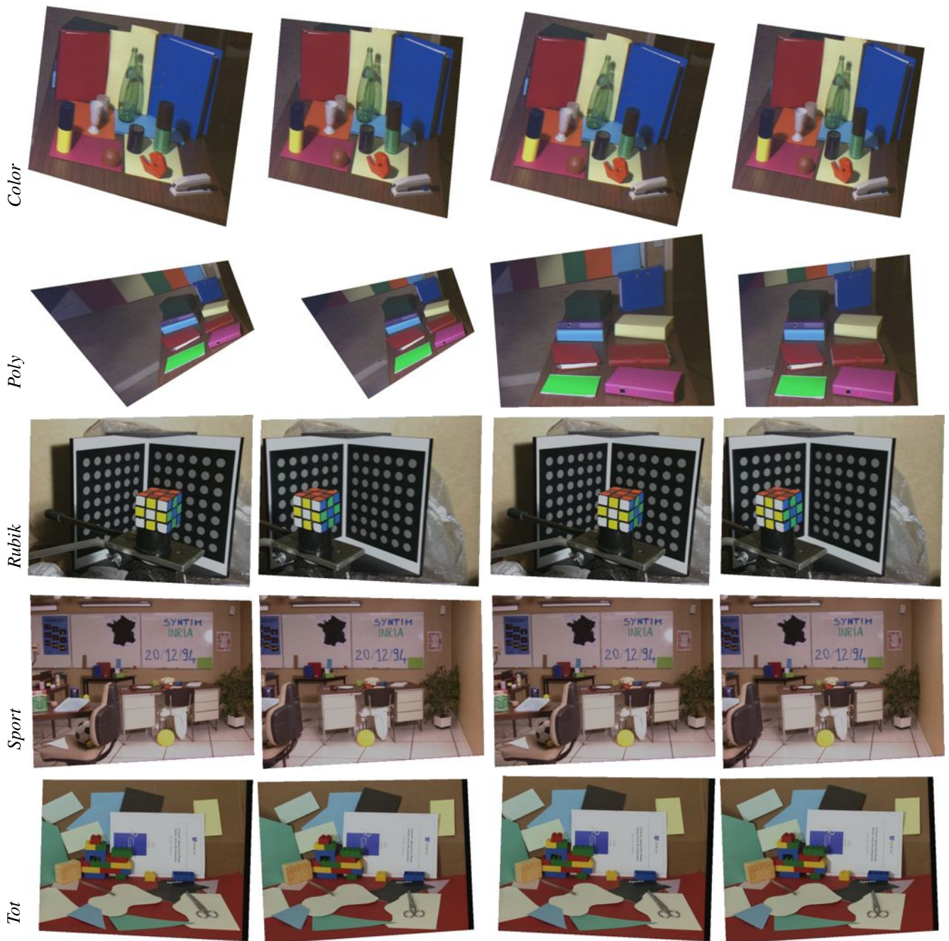
Figure 2. Euclidean (left) and quasi-Euclidean rectification (right) of the SYNTIM pairs.
