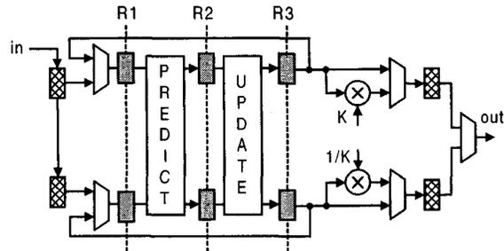
Fig. 5. Simplified block diagram with pre- and post-data formatter
