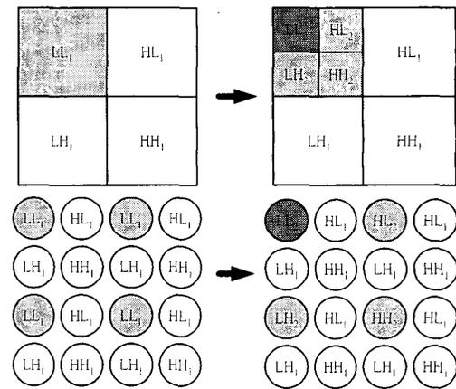
Fig. 8. Example of 2-level wavelet transform shows the in-place interleaving organization of wavelet coefficients, where a circle represents a pixel.
