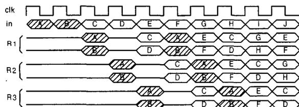
Fig. 6. Interleaving computation concept of the two stage operation in 9/7 filter mode
