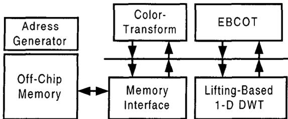
Fig. 9. JPEG 2000 system block diagram
