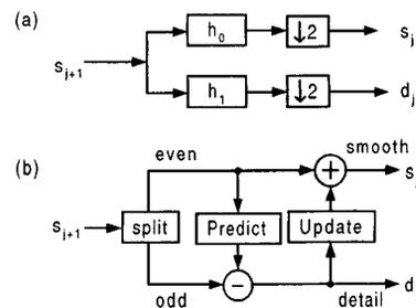
Fig. 1. Wavelet Transform: (a) classical implementation, (b) lifting-based implementation
