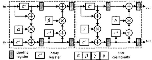
Fig. 3. Lifting based DWT architecture proposed in [10]
