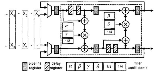
Fig. 4. Proposed folded architecture for 5/3 and 9/7 filter of DWT
