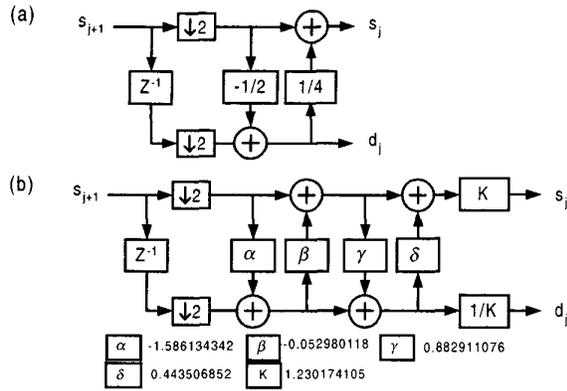
Fig. 2. Lifting-based implementation: (a) 5/3 filter architecture. (b) 9/7 filter architecture
