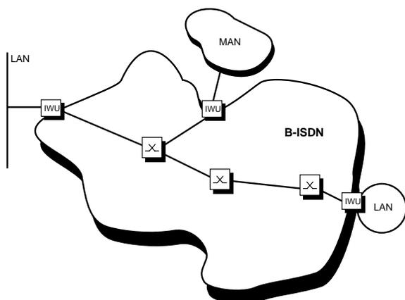
Figure 1: The indirect approach to connectionless service
