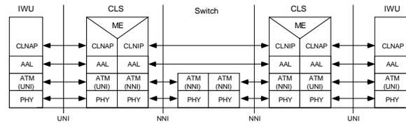
Figure 3: A direct approach protocol architecture
