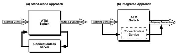
Figure 4: Stand-alone and integrated connectionless servers
