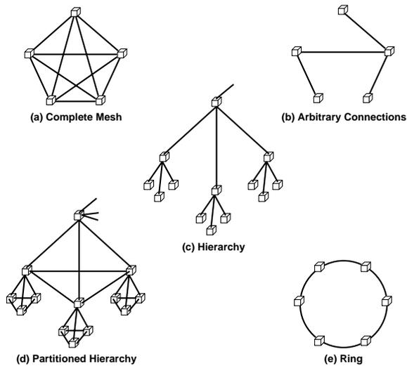
Figure 5: Connectionless server network topologies
