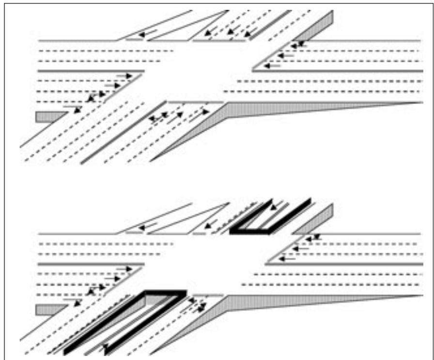
**Figure 1. At-grade intersection and prototype low-clearance underpass.**
