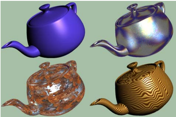
Figure 3: Images generated with the simple Blinn-Phong shader, two parameter settings for the encapsulated Blinn-Phong shader, and the wood shader derived using shader algebra operators. See Listings 1, 2, and 3.
