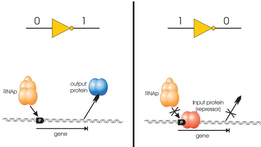
Figure 5: The two idealized cases for a biological inverter. If input repressor is absent, RNAP (RNA polymerase) transcribes the gene for the output protein and enables its synthesis. If input repressor is present, no output protein is synthesized.
