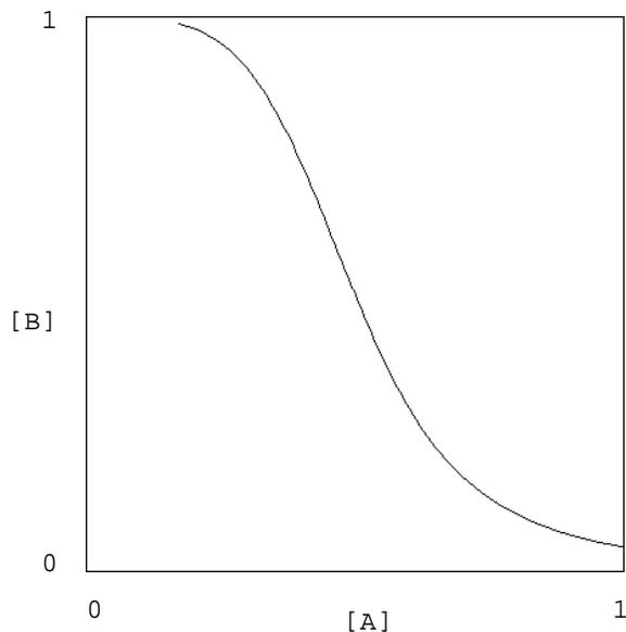
Figure 6: The DC transfer curve for the “inverter” that operates on DNA-binding proteins is similar to the input-output transfer characteristic of a digital inverter. The model of the chemical kinetics employed here postulates that four molecules of the repressor protein are required to inhibit production of the output.
