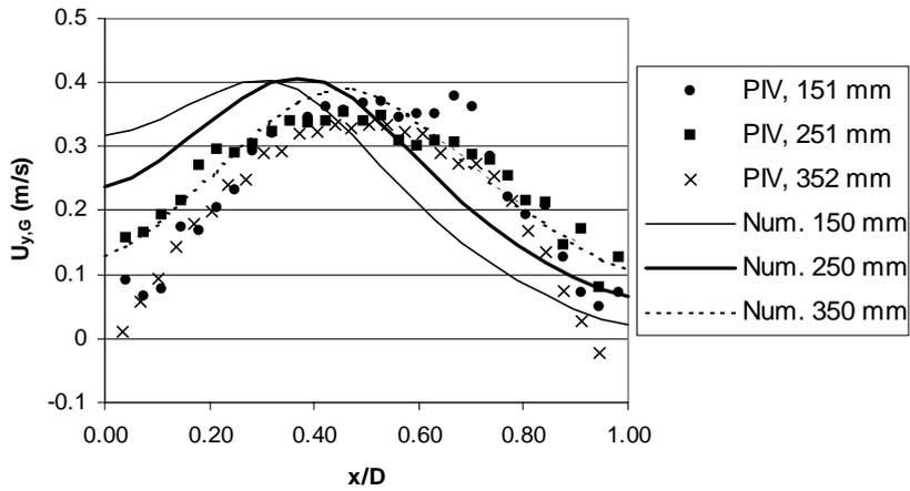
Fig. 9. Time averaged plot of the axial velocity component of the liquid phase at different heights in the column.
