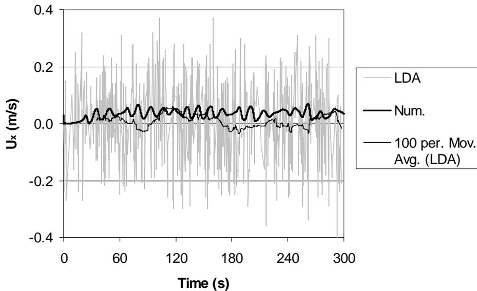
Fig. 7. Time plot of the radial velocity component of the liquid phase at a point on the centreline of the column,  $x = 0.075$ ,  $y = 0.075$ ,  $z = 0.250$ .
