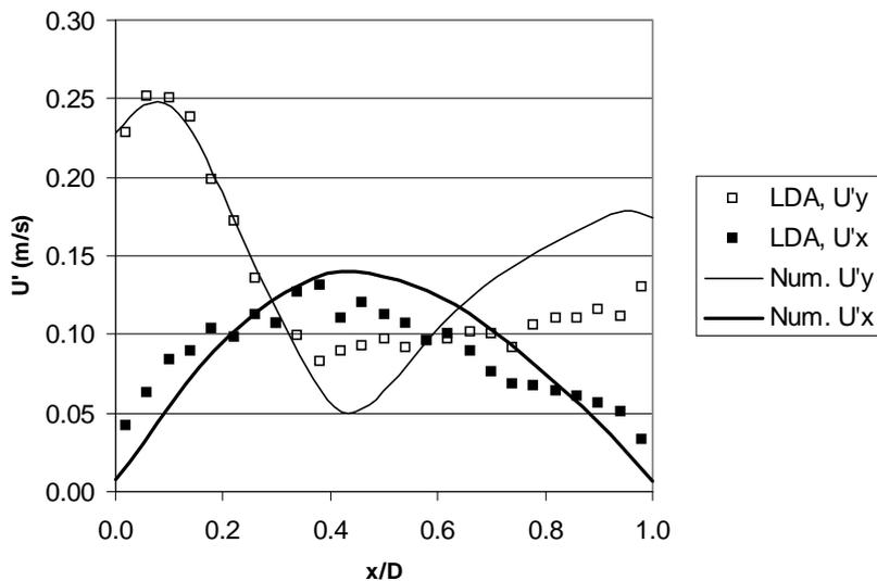
Fig. 4. Time averaged plot of the axial and radial velocity fluctuations of the liquid phase at  $y = 0.040$  m,  $z = 0.800$  m.
