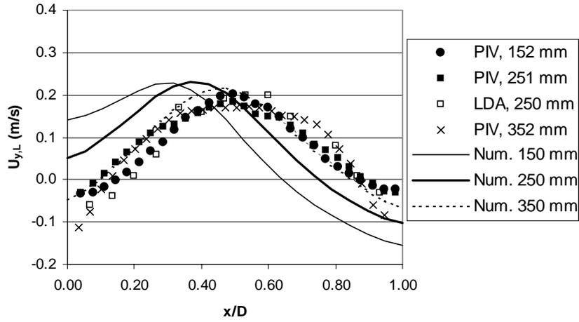
Fig. 8. Time averaged plot of the axial velocity component of the liquid phase at different heights in the column.
