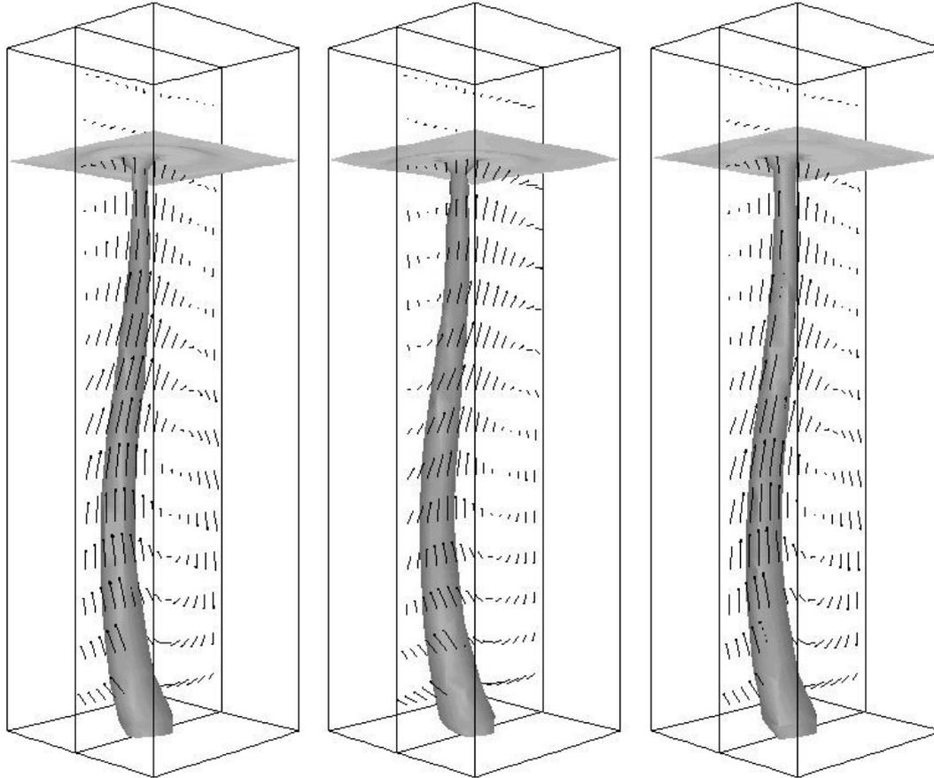
Fig. 5. Three snapshots of the iso-surface of the bubble plume in case h (i.e. the surface indicates  $\epsilon_G = 0.1$ ). The liquid velocity field in the centre plane is also shown. The plots are respectively 100, 200 and 300 s after the start of the simulation.
