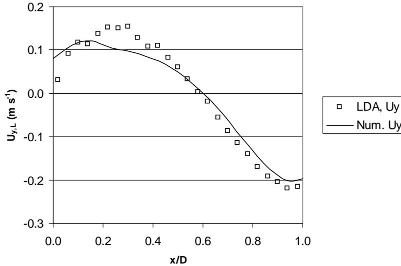
Fig. 3. Time averaged plot of the axial velocity component of the liquid phase at  $y = 0.040$  m,  $z = 0.800$  m. Experimental data by Becker et al. (1994).
