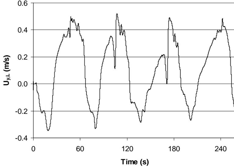
Fig 2. Time plot of the axial velocity component of the liquid phase at one point in the bubble plume,  $x = 0.035$  m,  $y = 0.040$  m,  $z = 0.900$  m.
