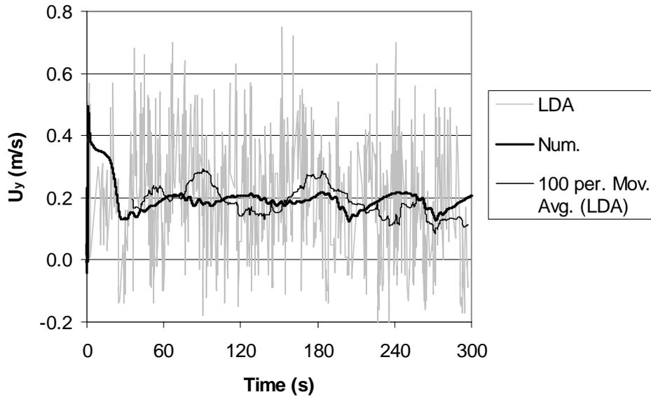
Fig. 6. Time plot of the axial velocity component of the liquid phase at a point on the centreline of the column,  $x = 0.075$ ,  $y = 0.075$ ,  $z = 0.250$ .
