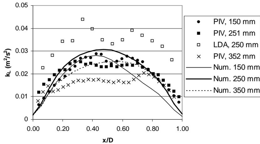
Fig. 10. Time averaged plot of the time averaged turbulent kinetic energy of the liquid phase at different heights in the column.
