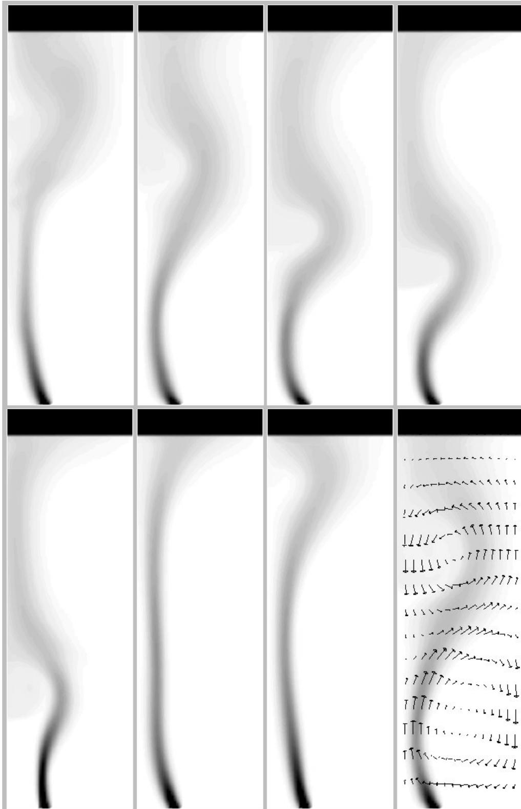
Fig. 1. Plots of the volume fraction of the gas phase,  $\epsilon_G$  at eight different instances, with time intervals of 10 s. White corresponds to  $\epsilon_G = 0$  and black to  $\epsilon_G > 0.05$ . The last plot also shows the velocity field of the liquid phase.
