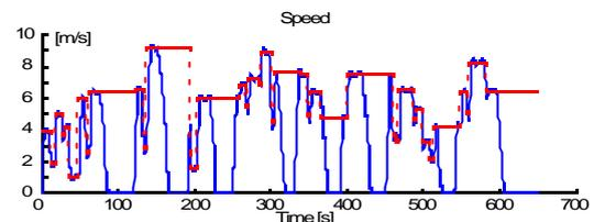
Fig. 11 "Speed Limit" and speed for a simulation including eight bus stops over 2.5 km.
