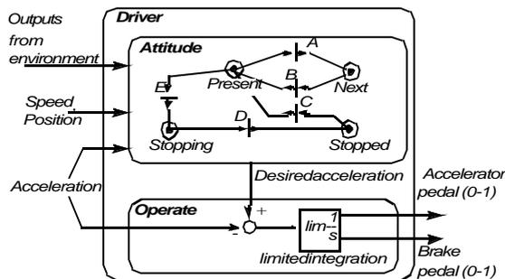
Fig. 15 Principles of the driver model.
