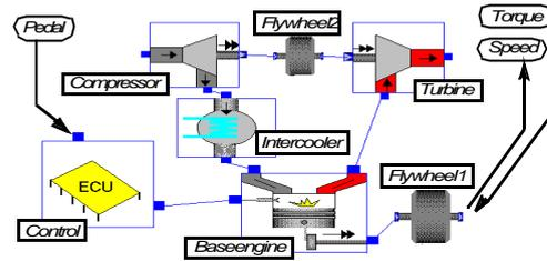
Fig. 16 Computer screen dump of ICE model with its natural causality shown by the arrows.
