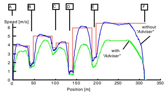
Fig. 10 The plot shows the result from a simulation where a bus is driven between two bus stops.
