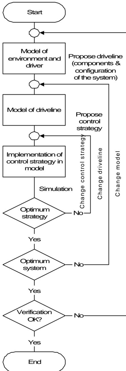
Fig. 1 Design process for a propulsion system.
