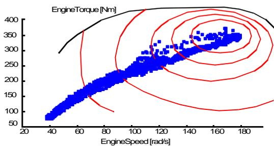
Fig. 7 Simulated conditions for the diesel engine when using the “Continuous control strategy”.
