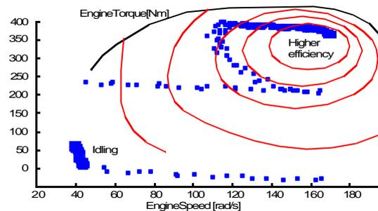
Fig. 6 Simulated conditions for the diesel engine when using the “On-Off control strategy”. Approximated values for maximum torque and constant efficiency lines for steady-state condition are also shown.
