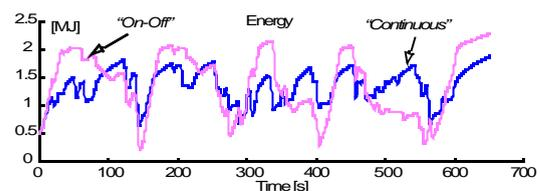
Fig. 12 The energy in the storage unit for the "On-Off" and the "Continuous" control strategy.
