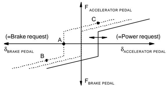
Fig. 19 The principal characteristics of the adjustable accelerator- and brake pedals.
