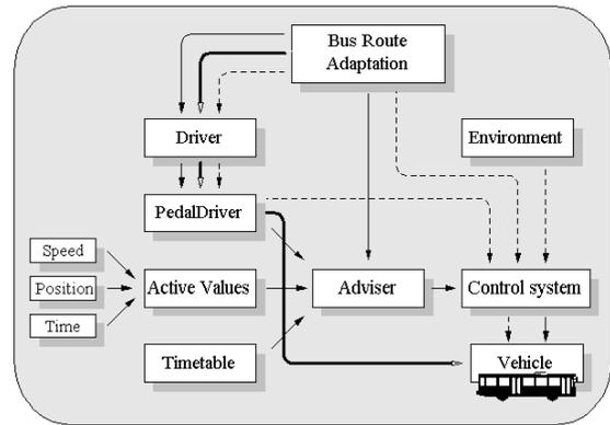
Fig. 3 Information flow for bus route adaptation. The thick line shows the condition for a conventional bus, where only the bus driver has information of the route and time table. The information flow for the “Adviser” is marked with narrow lines and the “Adapter” concept with dashed lines.
