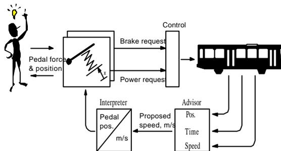
Fig. 18 Driver indirectly affects the control system of the vehicle and the advisor gives force and pedal position feedback via an interpreter.
