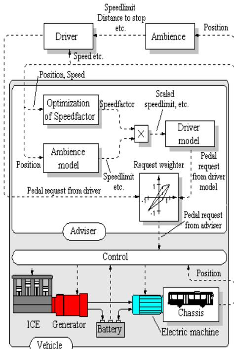
Fig. 8 Layout for the information flow for the whole simulated system.
