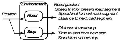
Fig. 14 Principles of the environment model.
