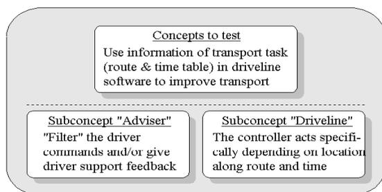
Fig. 2 Concepts of this work. The first one, which is called subconcept “Adviser”, is like a filter that helps the driver to drive in an efficient way. The second one utilizes directly the information on the transportation task to control the propulsion system, without affecting driver.
