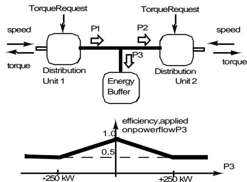
Fig. 17 Model of energy distribution and buffering system.
