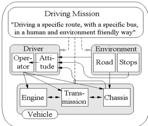
Fig. 4 The natural causality for a conventional city bus. The “Driving mission” gives input to the driver in the form of route, time table and what vehicle to use. When the driver performs the mission, his “Attitude” part makes decisions which are carried out by the “Operator” part. The response of the vehicle is registered by the driver. The environment affects the vehicle as well as it gives input to the driver in form of suitable speed and positions where to stop.
