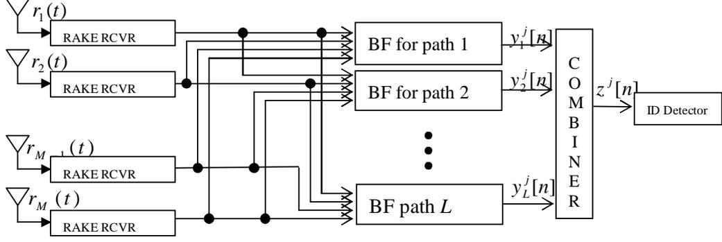
Fig. 4. DBS(TRX) receiver structure assuming a frequency selective channel and smart antennas with DS-CDMA
