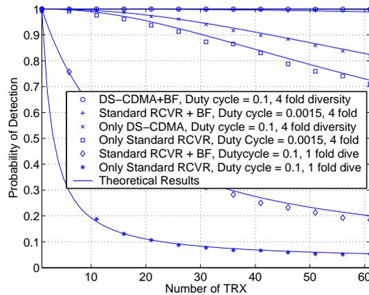
Fig. 5. Simulation results for DBS receivers, without perturbation.
