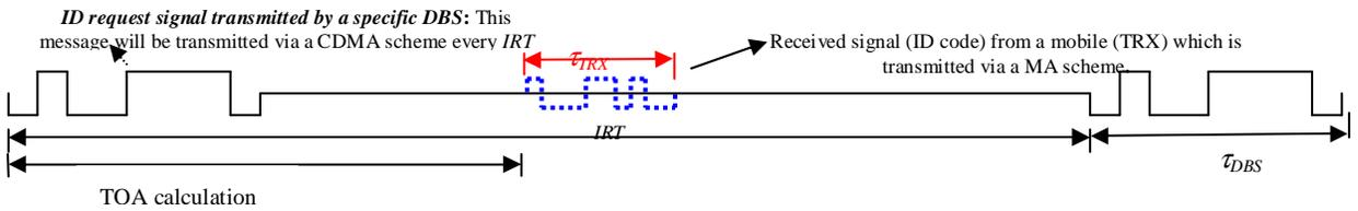
Fig. 1. Transmission of IDR and reception from TRX in DBS. Assuming a Pseudo Random ID codes, the number of the bits in the code represents the maximum capacity of the WLPS.
