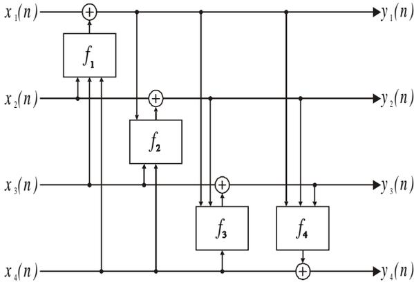
Figure 1: Four-band filter structure.
