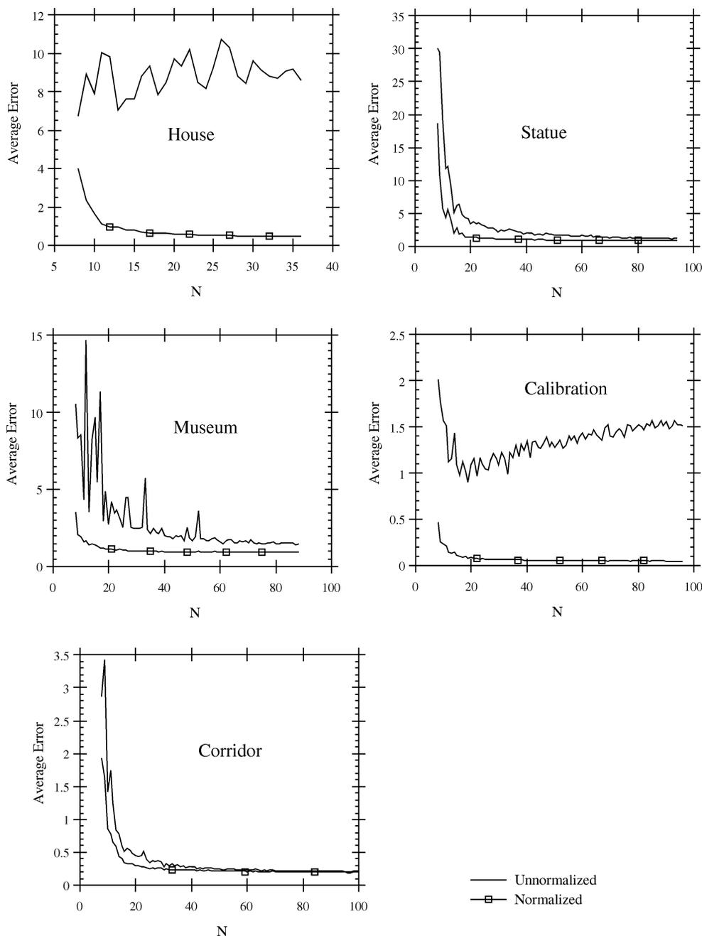
Fig. 8. Comparison of normalized and unnormalized eight-point algorithms.
