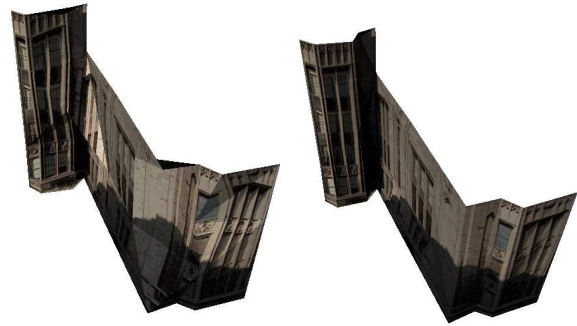
Figure 10: The triangulated surface created from a 2D Delaunay triangulation (left) and our refined triangulation (right).
