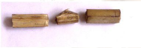
Fig 7 Failed bamboo samples in shear test
