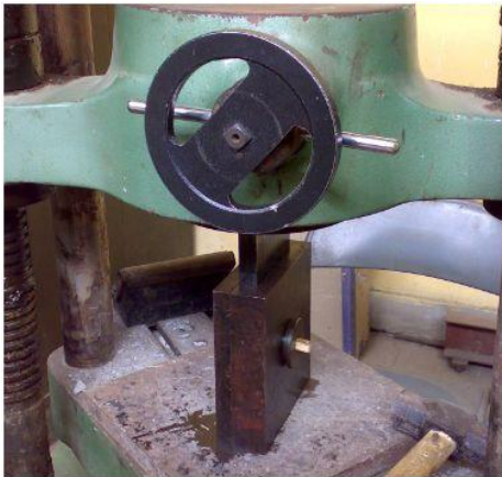
Fig. 3 Test setup of Shear shackle arrangement in U.T.M
