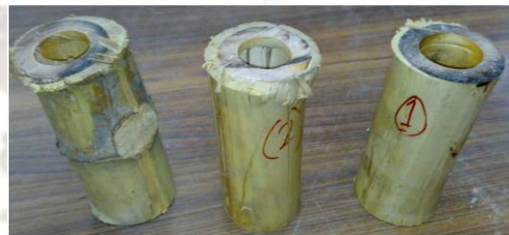
Fig 6 Failed bamboo samples in compression test
