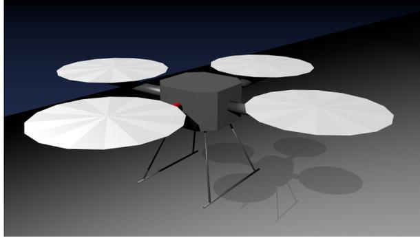
Figure 2: This is the quadcopter model provided by `hector_quadrotor` for simulation in Gazebo, dubbed “HERP” for the purposes of these experiments. Rendering from [5].
