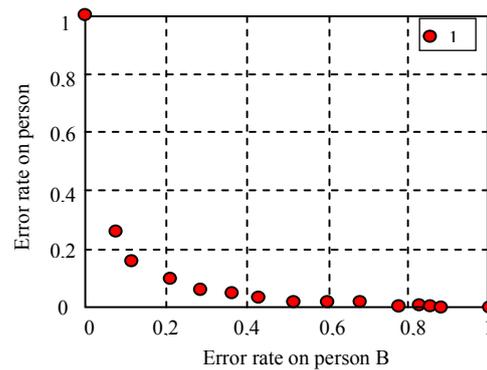
Fig. 2 The ROC curve with error rates for fingerprint identification subsystem
