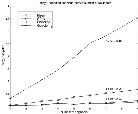
Figure 11: Energy dissipation versus node degree.
