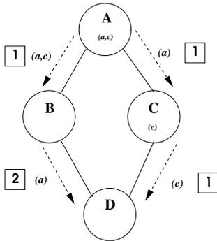
Figure 5: Ideal dissemination of observed data  $a$  and  $c$ . Each node in the figure is marked with its initial data, and boxed numbers represent the order in which data is disseminated in the network. In ideal dissemination, both implosion, caused by B and C's common neighbor, and overlap, caused by A and C's overlapping initial data item,  $c$ , do not occur.
