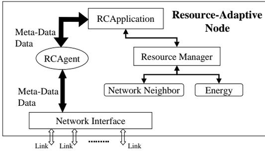
Figure 6: Block diagram of a Resource-Adaptive Node.
