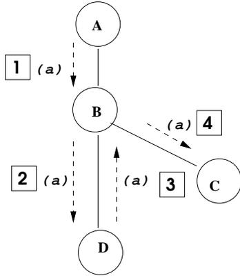
Figure 4: Gossiping. At every step, each node only forwards data on to one neighbor, which it selects randomly. After node D receives the data, it must forward the data *back* to the sender (B), otherwise the data would never reach node C.
