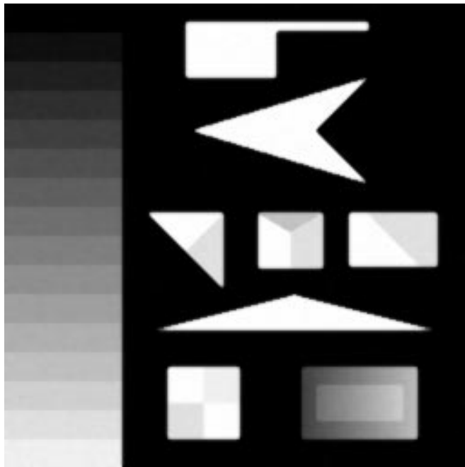
Figure 35: The result of applying K -nearest neighbour filtering to the noisy image.
