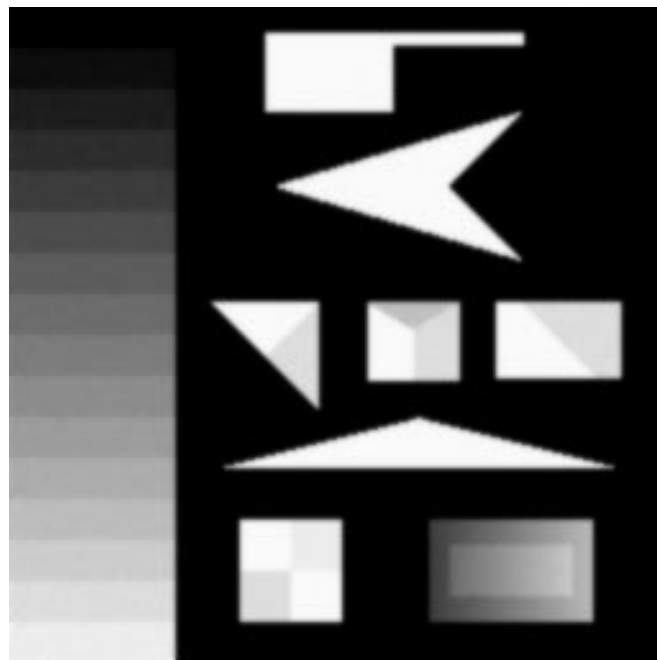
Figure 31: The result of applying Gaussian filtering with \sigma = 1.0 to the noisy image.
