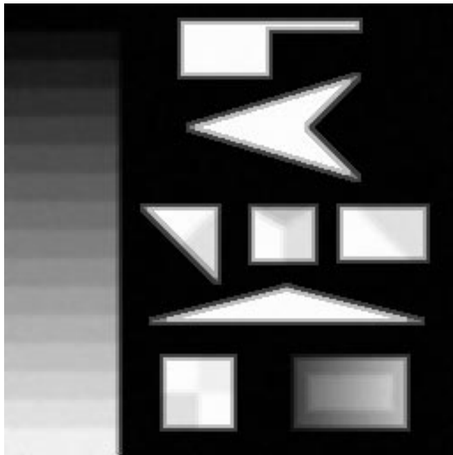
Figure 33: The result of applying midrange filtering to the noisy image.
