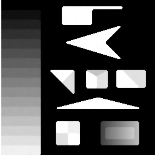
Figure 32: The result of applying median filtering to the noisy image.
