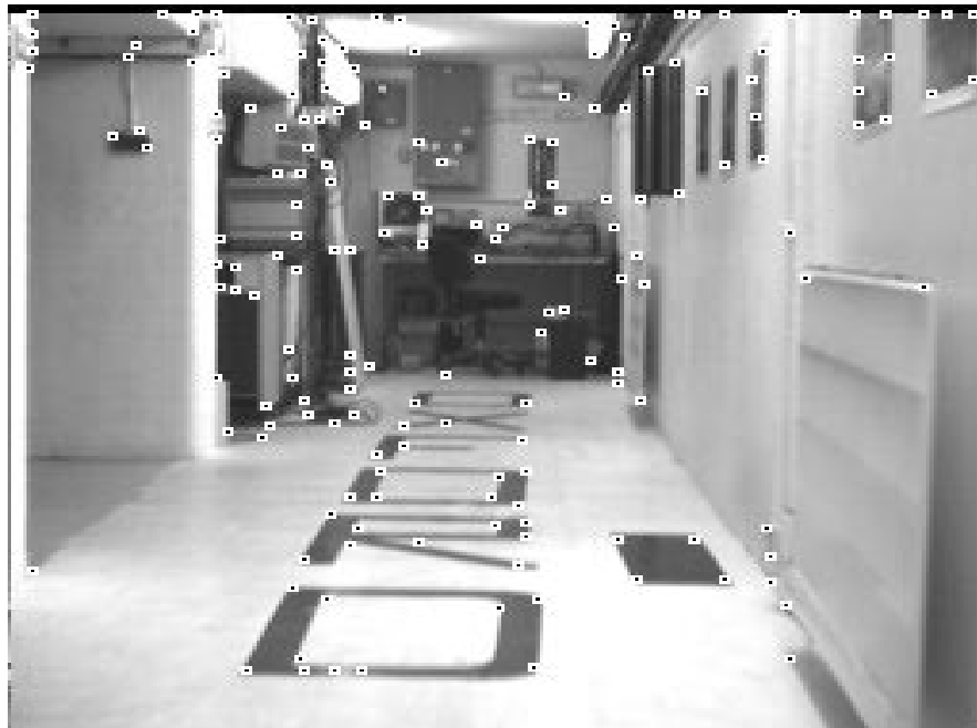
Figure 27: Output of the SUSAN “corner” finder ( t=25 ) given a real image captured by video camera.
