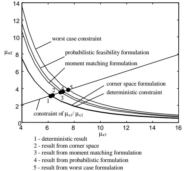
Figure 6. Results of the Beam Example
