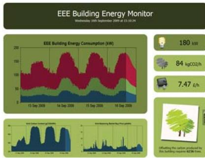
Figure 1: Live information screen displaying energy and carbon emission data for a building at the University of Southampton (see <http://energy.ecs.soton.ac.uk/energy/>).
