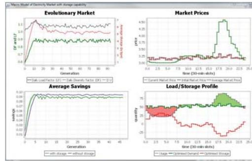
Figure 3: Java simulation of a smart grid incorporating micro-storage showing the flattening of the aggregate demand profile (see <http://users.ecs.soton.ac.uk/pv/simulator/storage/storage.mp4>).
