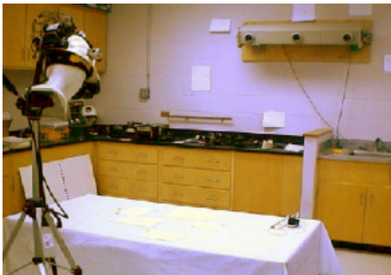
Figure 11 Real motion experimental setup, with Optotrak sensor on wall.
