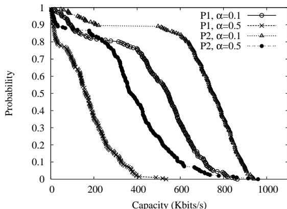
Fig. 2. The distribution of the end-to-end capacity on two separate path of a fixed density  $\rho^{(i)}$  and  $\rho^{(j)}$  while modifying  $\alpha$  the activity factor of the primary nodes.
