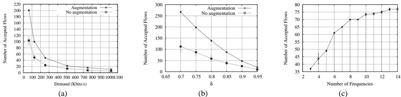
Fig. 3. The number of accepted connections for different  $D$  in (a), reliability levels ( $\delta$ ) in (b) with and without augmentation, and the number of used channels with augmentation (c).
