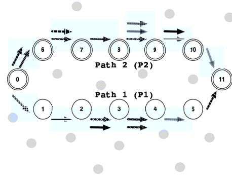
Fig. 1. Two simulated topologies showing the two paths from node 0 to node 11. Path 1 (P1) goes through node 1 while Path 2 (P2) through node 6
