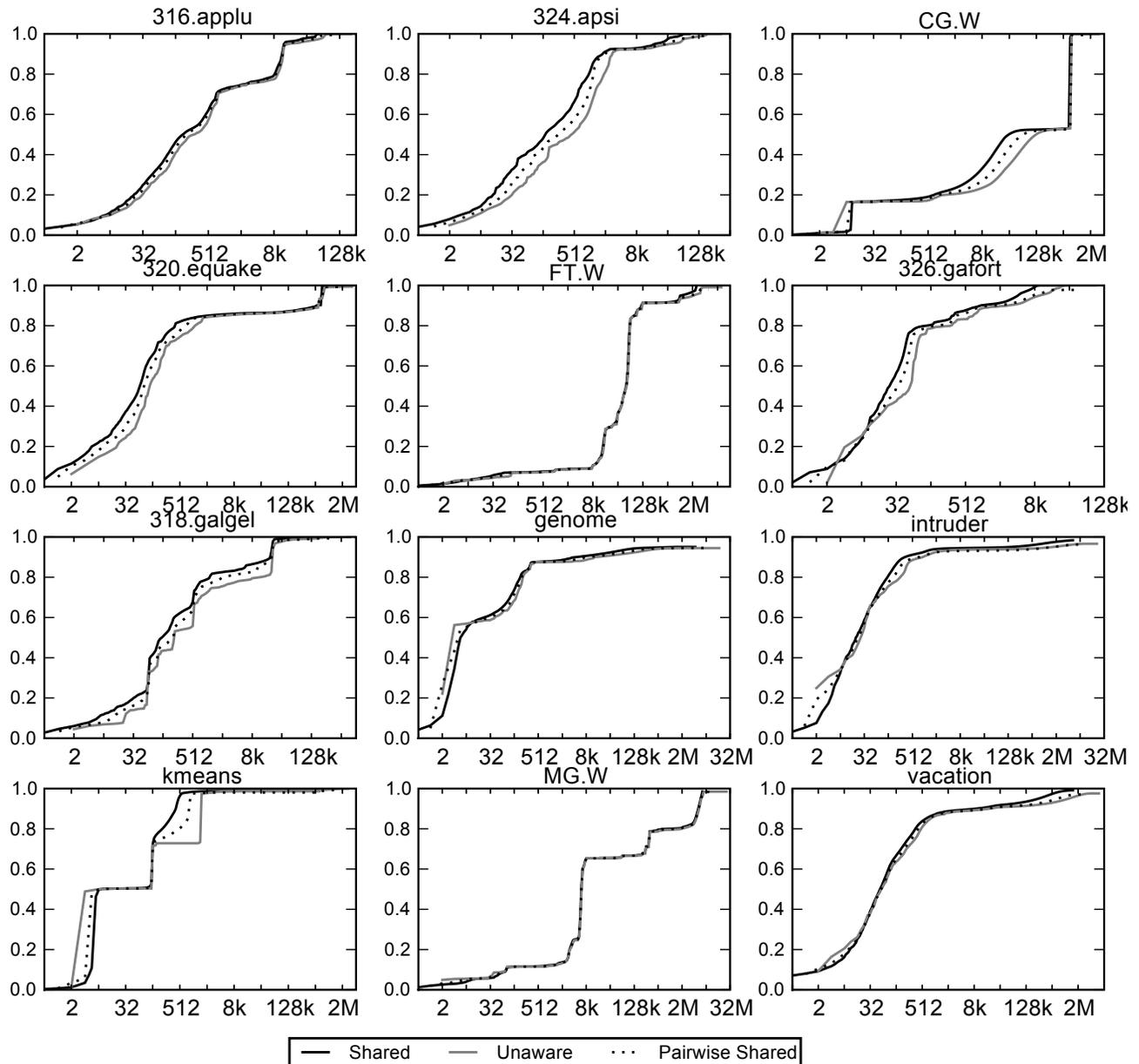
Figure 2. CDFs of reuse distance using a single shared or pairwise shared stacks. X axis is reuse distance in 64-bit words, Y axis is fraction of references with reuse distance less than  $x$ .
