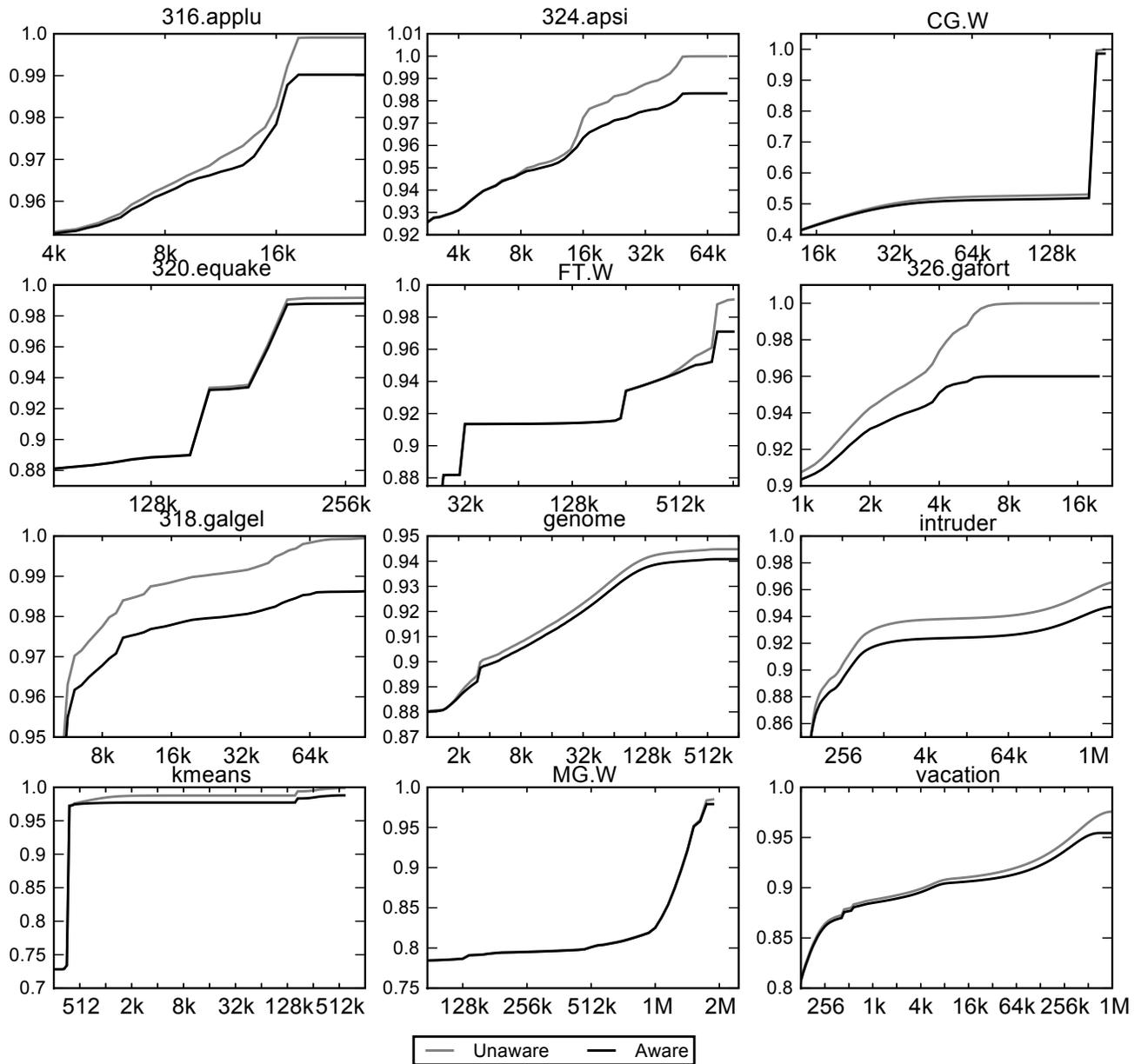
Figure 1. CDFs of reuse distance using private per-thread stacks. X axis is reuse distance in 64-bit words, Y axis is fraction of references with reuse distance less than  $x$ .
