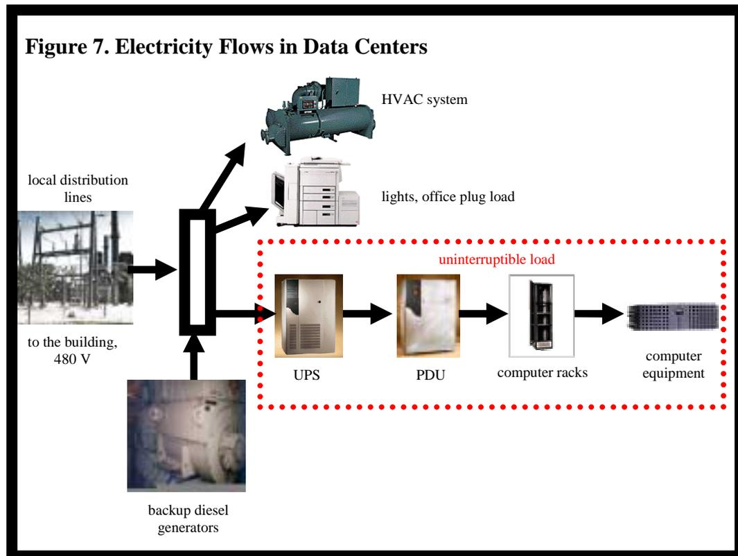
computer equipment will lose power. While it is possible to feed the racks of computer equipment directly from the AC grid while making sure that the battery is charged, in this type of system a power outage might cause the computer equipment to lose power for a fraction of a cycle while the power source switches from the grid to the batteries.
