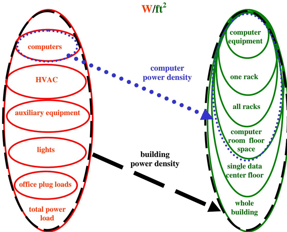
Data center designers indicate that the majority of existing data centers have a *design* computer power density of 50 to 75 W/ft<sup>2</sup>.<sup>37</sup> Despite reports from facility managers that actual power densities are less than design, the companies building data centers have started to request much higher power densities and thus designers have begun to create data centers that can accommodate 100 to 150 W/ft<sup>2</sup> computer equipment loads in this central computer space.
