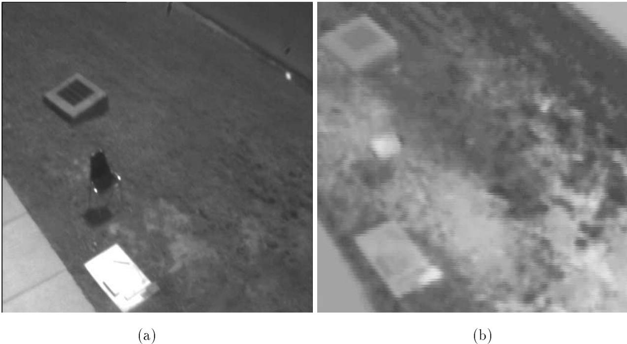
Fig. 7. (a) A visual image of the scene used for these experiments. Materials include Asphalt, Concrete, Dirt, Fiberglass, Iron, Slate, and Wood. (b) A corresponding long-wave infrared (LWIR) image. The scene was imaged at 7 different times over a 2 day period.
